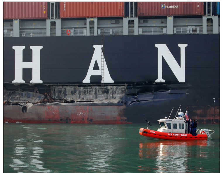
Hole in the Cosco Busan container ship, which spilled 53,000 gallons of oil in San Francisco Bay in 2007.
