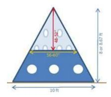
Figure 8-5. An example of the predesigned pyramid structures with the open side.
