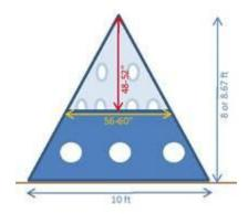
Figure 8-16. An example of the predesigned pyramid structures with the open side.
