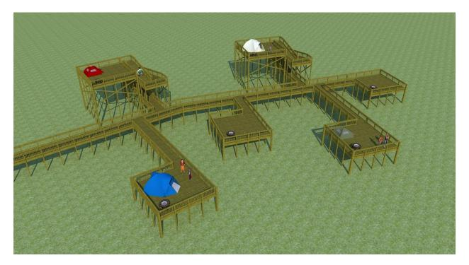
Figure 8-39. Artist's vision of a possible design for tent camping platforms at Galveston Island State Park. Graphic created by Richard Garcia, TPWD Infrastructure Division, Planning and Design Branch.
